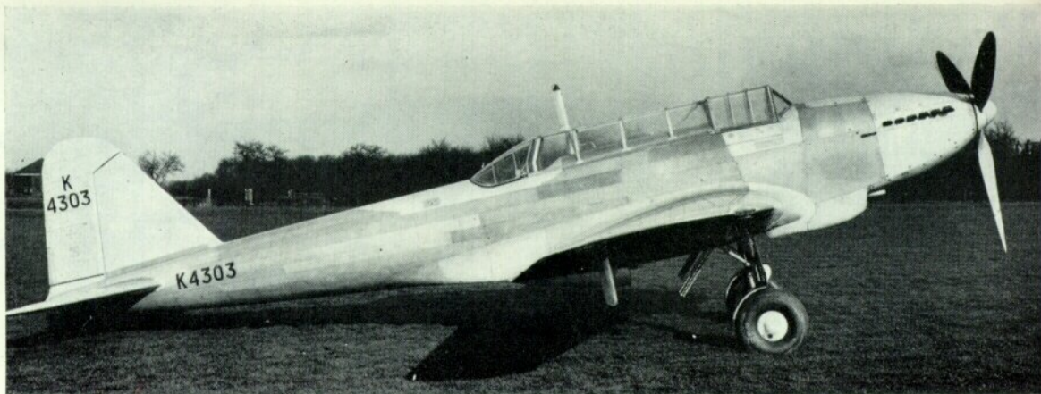
Battle prototype K4303 with original cockpit canopy.
